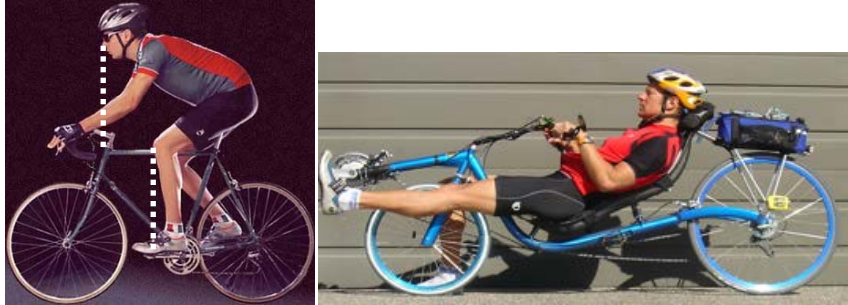
Figure 1: The differences in design and posture associated with a standard diamond framed road bike (left) and a recumbent bike (right). Images from http://www.jimlanglev.net (left), http://venturecyclist.blogspot.co.uk (right).
