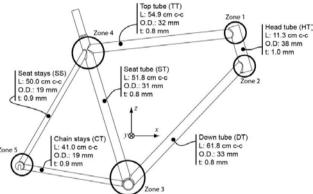
Fig. 1. Details of the frame/tube geometries for the road bicycle frame analysed in this study (head tube angle XX°, seat tube angle YY°).
