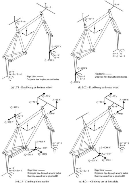
Fig. 2. Free body diagrams for the four load cases simulated in this study, based on measurements presented in the literature. Note  $\theta_{\text{crank}}$  is measured anticlockwise from the vertical *z*-axis.
